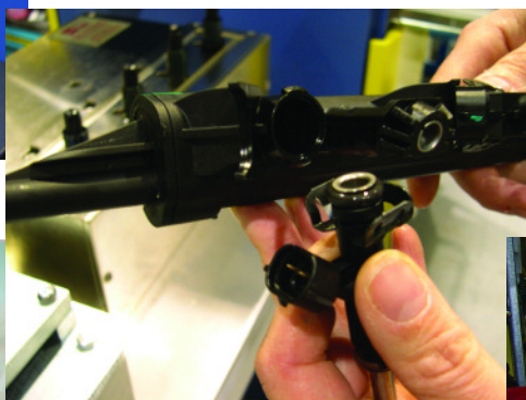
Assembling the injector into the fuel rail
