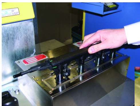
Placing the fuel rail in the lubricating fixture
