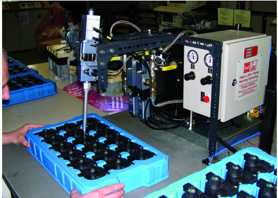
Metering the mixed silicone onto the assembled PCB's.
