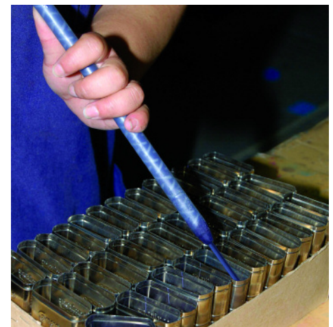
Dispensing the mixed epoxy resin into the paint brush ferrules via a disposable plastic static mixer
