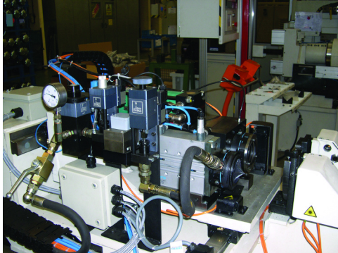
Electronic flowmeter grease metering module
